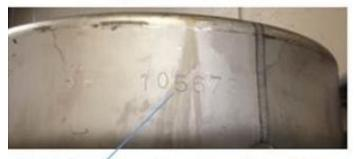
Can be found in various places (depending on manufacture date, etc.) but always etched into the stainless. Permanent part of the keg.
